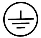
terminal is for equipment grounding only. **Enclosures**
