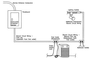
Arc-fault Scenario **Protection Provided Branch-circuit Wiring** Parallel Arcing Detection Series Arcing Detection Υ (With Ground) Series Arcing Detection Υ Without Ground (#) Cord Sets (Extension Cords), Power-supply Cords Parallel Arcing Detection Series Arcing Detection
