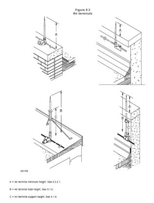
A= 10 inches minimum height B= 24 inches or more in height C= support shall be located at not less than one half the height of the terminal
