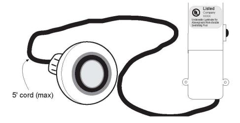
Fig. 3 - Underwater Luminaire for aboveground storable swimming pool.
