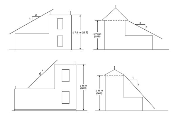
SECONDARY ROOF AREA – A secondary roof is less than 10 percent of the total roof area of the protected building and lower than adjacent roofs.
